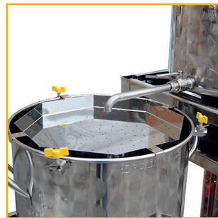
Fly sparge installé
