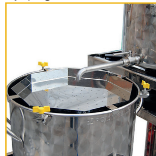
Fly sparge installé
