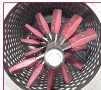
Destemming shaft with rubber-coated paddles.
