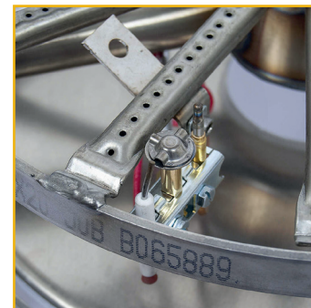
Piezoelectric Unit, Safety, Pilot Flame
