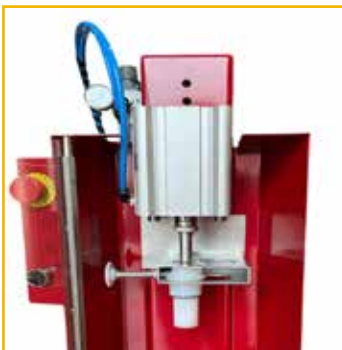
Cone for inserting a cork cap
