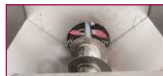
Hopper interior with stainless steel auger
