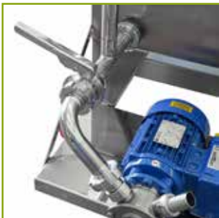
Inlet/Outlet Control Valves
