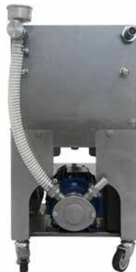
Pump with nitrile impeller
