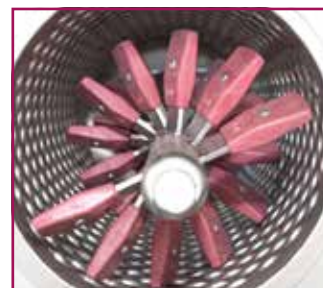
Destemming shaft with rubber-coated paddles.
