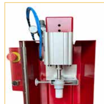
Cone for inserting a cork cap
