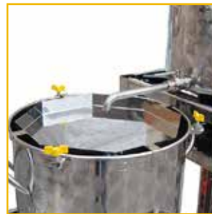
Fly sparge installé
