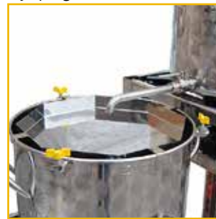
Fly sparge installé
