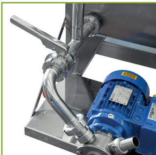
Inlet/Outlet Control Valves
