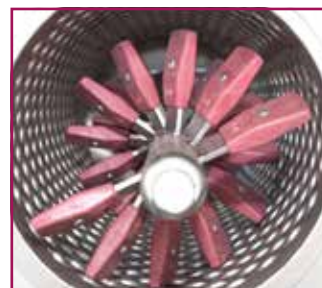
Destemming shaft with rubber-coated paddles.
