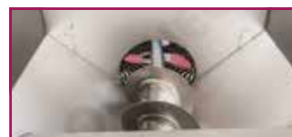
Hopper interior with stainless steel auger
