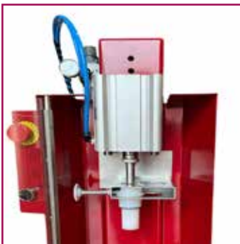
Cone for inserting a cork cap
